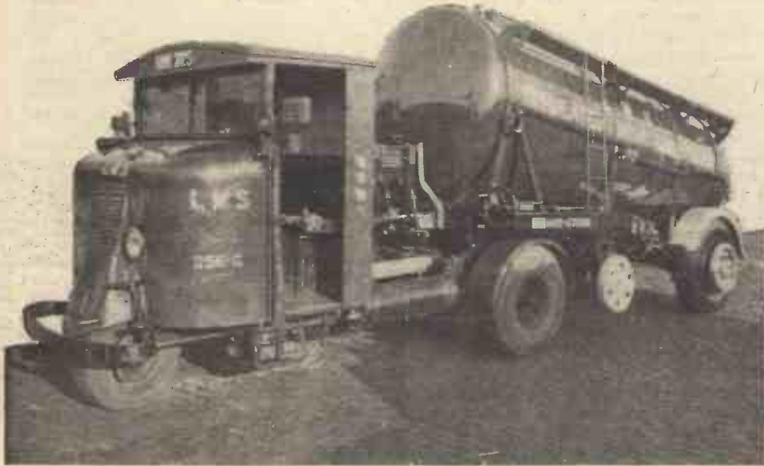
The new edible-oil tank connected to a motor, and ready for transport by road.
