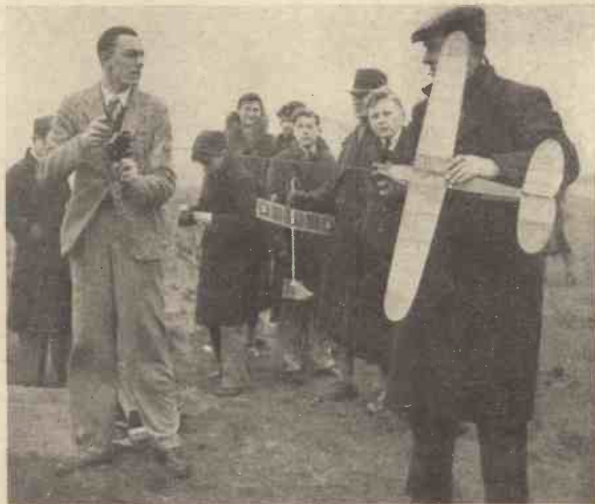
Winding a rubber motored model with the aid of a winder made from a bench grinder, at a recent meeting of the Kingston and District Model Flying Club on Wimbledon Common. The practice of stretching the rubber whilst winding originated in America, and is being adopted in this country. It is claimed that a much greater number of turns can be placed on the rubber skein in this way.
