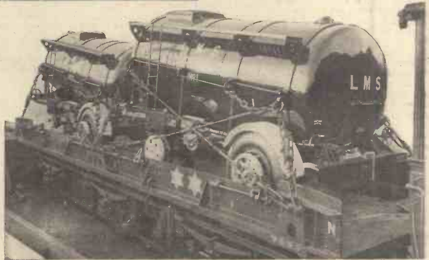
Two oil tanks on a specially constructed six-wheeled truck for transport by rail.
