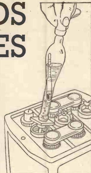
Fig. 1.—The method of testing an accumulator by means of a hydrometer. A reading of about 1.300 should be obtained when the battery is fully charged.
