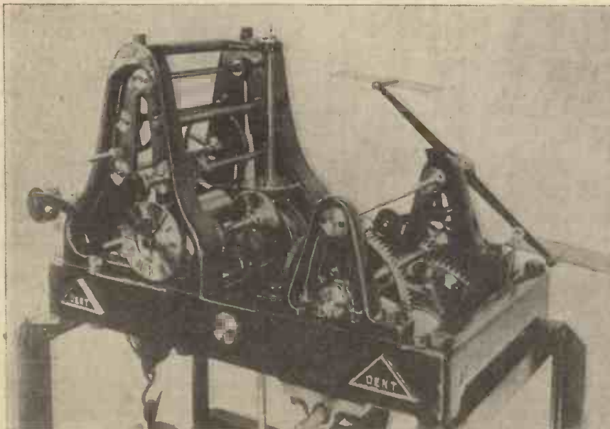
An example of up-to-date clock mechanism. The movement of a "turret" or tower clock, which is weight-driven and pendulum-controlled.
