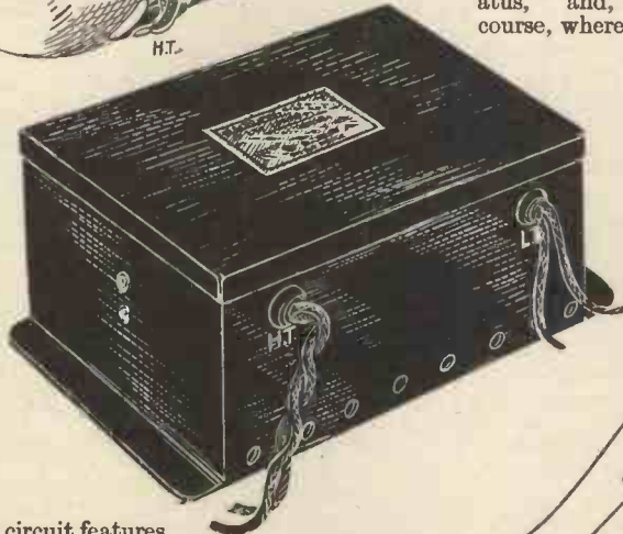
Fig. 1.—A rotary transformer which is a very useful type of unit. Below, the unit enclosed in a case.
