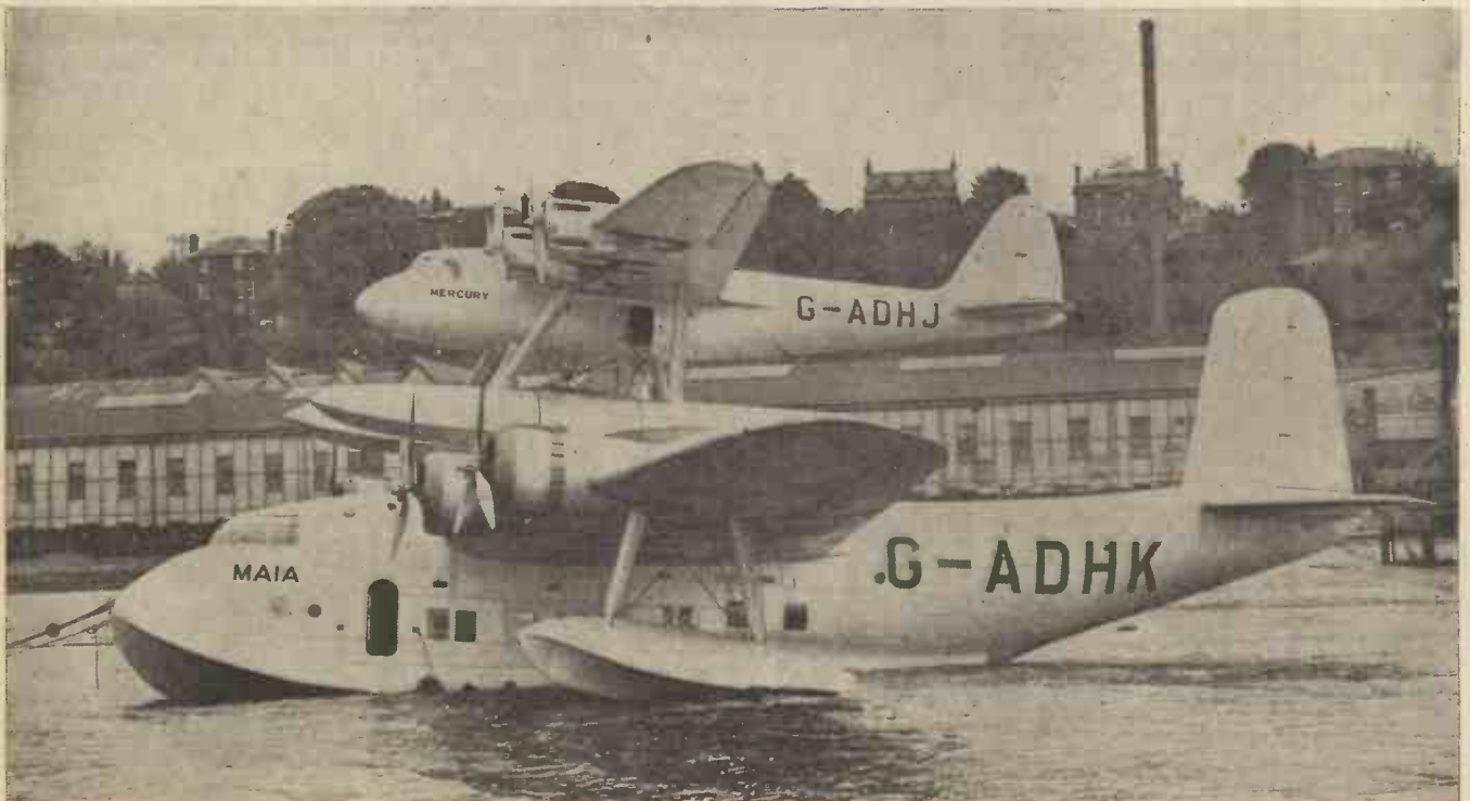
The ingenious pick-a-back aircraft designed by Imperial Airways to facilitate Atlantic flights.
