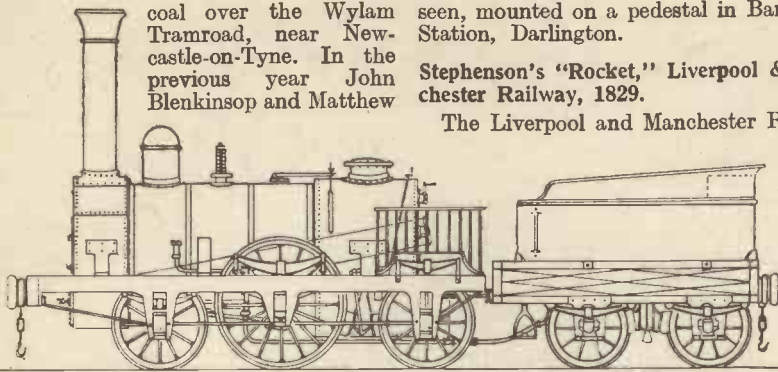
Robert Stephenson's "Patentee," 1834. The precursor of the single driver inside cylinder express locomotive.
