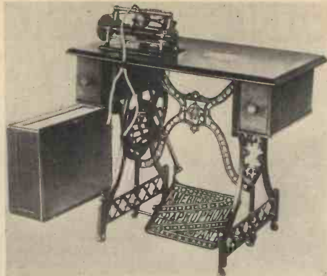
One of the earliest phonographs known. It was operated by a sewing-machine treadle.
