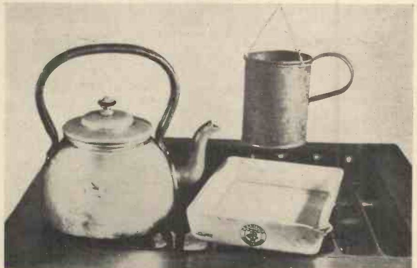
A simple method of obtaining distilled water for silvering operations. The steam from a kettle spout is directed against the outer sides of a suitably suspended vessel containing cold water, the condensed steam being collected in a vessel beneath.
