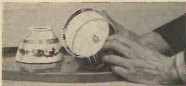
Fig. 1.—The china bowl here being shown has the rim ground flat and the mica disc illustrated fits on this ground rim, forming a lid which, when the bowl is filled with water, is kept in place by atmospheric pressure.
