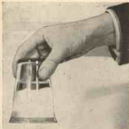
Fig. 6.—The water remains magically in the glass although the glass is held upside down. The presence of the mica disc seen in Fig. 5 accounts for this.
