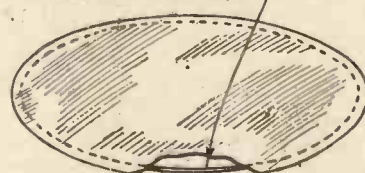
Fig. 9.—Disc of mackintosh with elastic in the hem. The elastic ring must be smaller than the diameter of the bowl so as to tightly fit over it. It is shown the same size here to make clear the construction of the cover.
