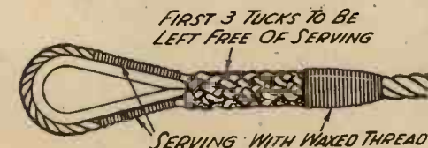
Fig. 24.—Showing the complete splice.
