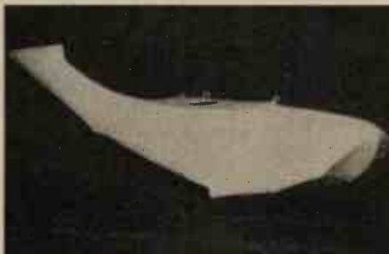
Fig. 10.—The flying-boat hull now covered with its \frac{1}{8} -in. sheet balsa and doped silk.
