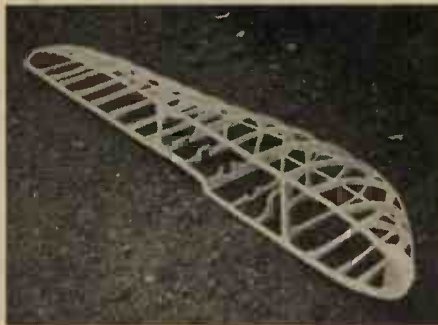
Fig. 6.—Captain Bowden's 30-c.c. racing hull half finished. One side is built on to a centre backbone of balsa wood.
