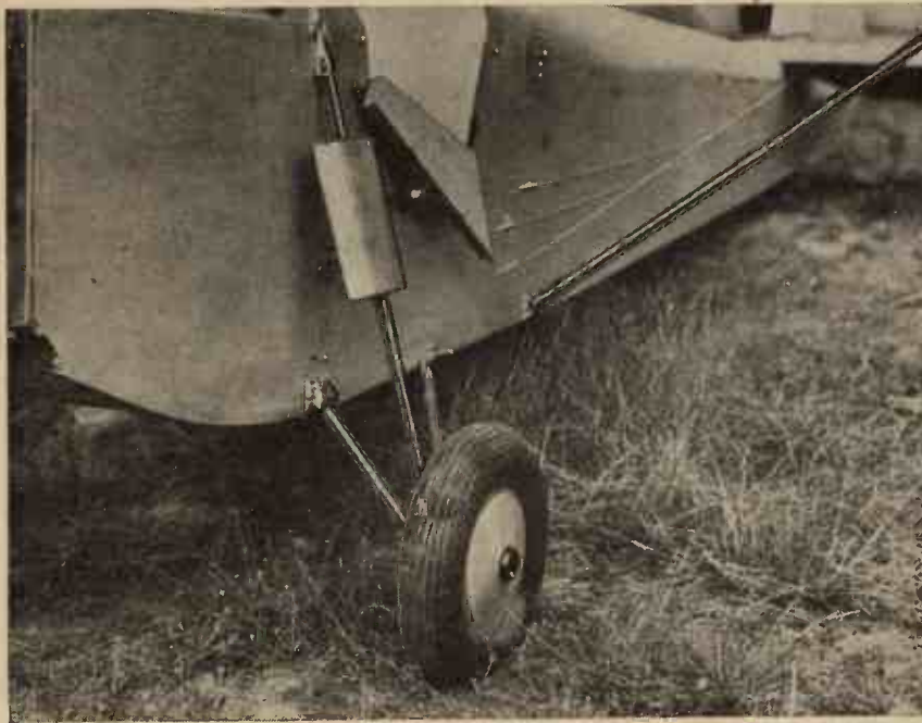
Fig. 18.—Showing the construction of the undercarriage.
