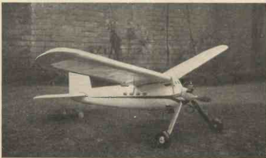
Fig. 1.—The writer's 6-c.c. model which has a 5 ft. 8 in. span and a monocoque fuselage.
