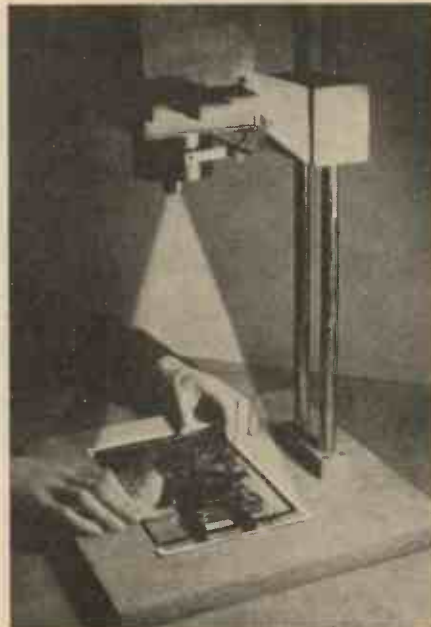
Fig. 2.—Just a clean sheet of glass, with strips of black paper gummed along each edge, will give a perfectly clean white border to the enlargement.
