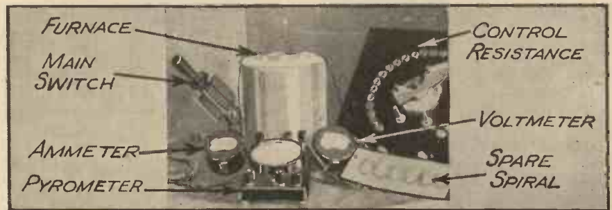
Fig. 2.—The general layout of the apparatus.
