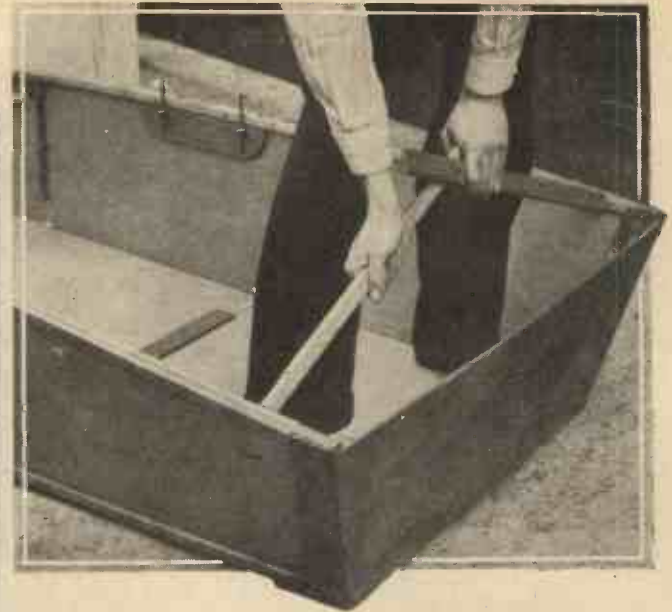
Fig. 7.—The sides of the boat are forced apart with the stretcher while the stern board and centre stretcher are placed in position.
