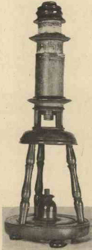
An early microscope of Hooke's day. It is made out of wood and cardboard.
