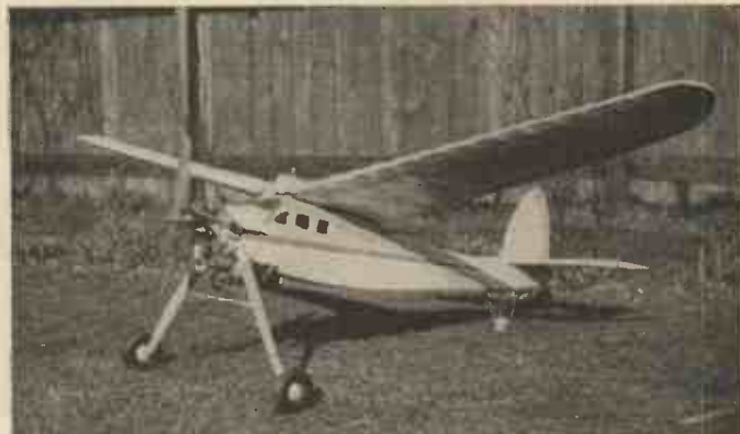
This photograph shows the 2.3-c.c. "Spitfire" mounted in the "Petrel."
