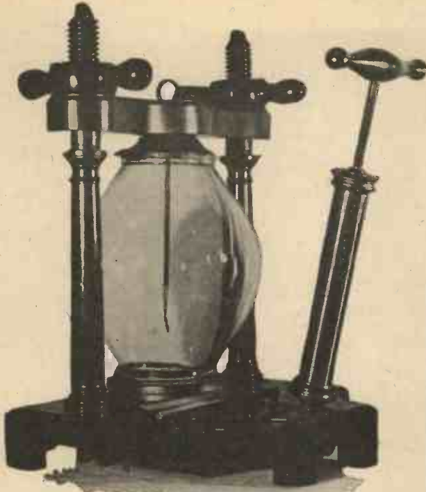
A premature vacuum pump of the type used by Hooke in his experiments.
