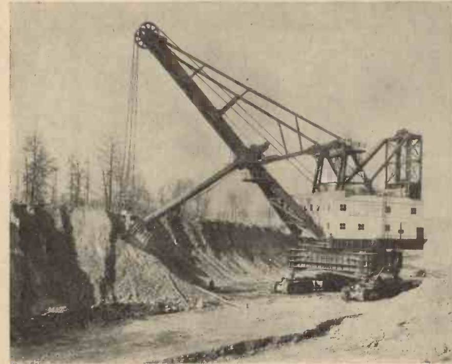
The world's largest electric shovel mounted on caterpillars, which weighs, in working order, 1,150 tons, and carries a dipper or bucket of 33 cubic yards capacity. This type of machine is used extensively in America for stripping the overburden of waste material off the coal deposits so that the coal may be mined, in the open without the necessity of costly underground tunnelling.
