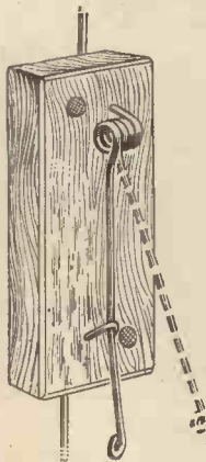
The first lighting switch.
