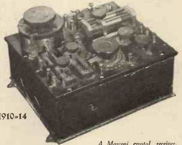
A Marconi crystal receiver, period 1910-14, as used in many ships' installations.
