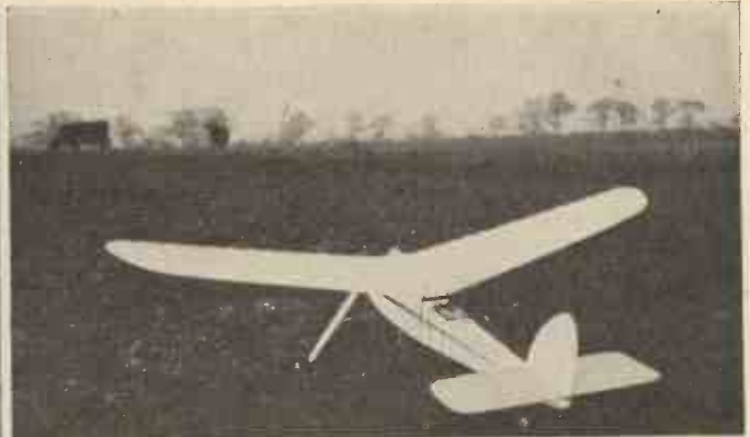
Fig. 2.—A three-quarter rear view of the model described showing the clock, and the petrol tank can be seen mounted into the wing.
