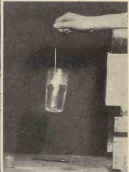
A spectacular experiment. A yale key tied to a piece of string has been cooled in liquid air and then immersed in a tumbler containing hot water. The key has frozen hard to the sides of the glass with the result that the entire tumbler of hot water can be lifted up and held in mid air. Note the coating of frost on the lower half of the string.
