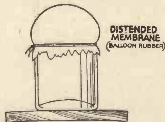
Fig. 4.—The expansion of ordinary air in space. The jam-jar contains air at ordinary pressure, which bursts the membrane as it expands.
