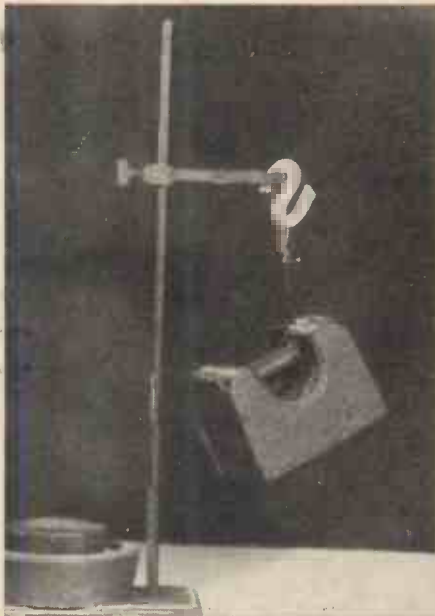
A hook of solid mercury suspending a 7-lb. weight. The mercury has been frozen in liquid air.
