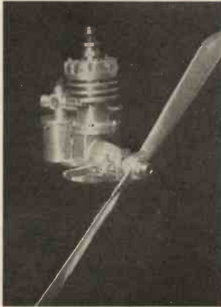
Mr. G. W. Macdonald's miniature engine which, under test, has achieved a speed of between 2,000 and 3,000 revolutions per minute.
