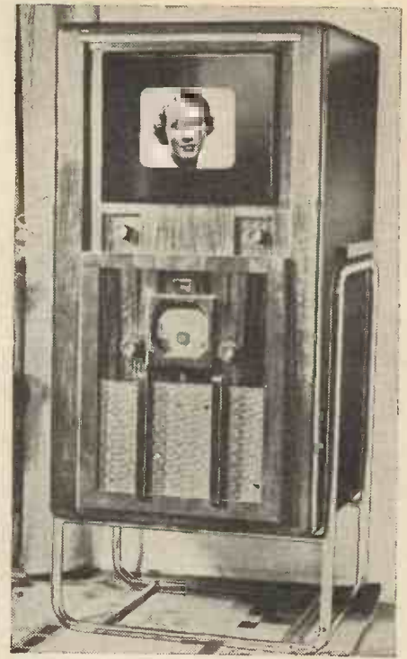
The Philips receiver is fitted to a neat chromium stand to increase the height of the viewing screen.
