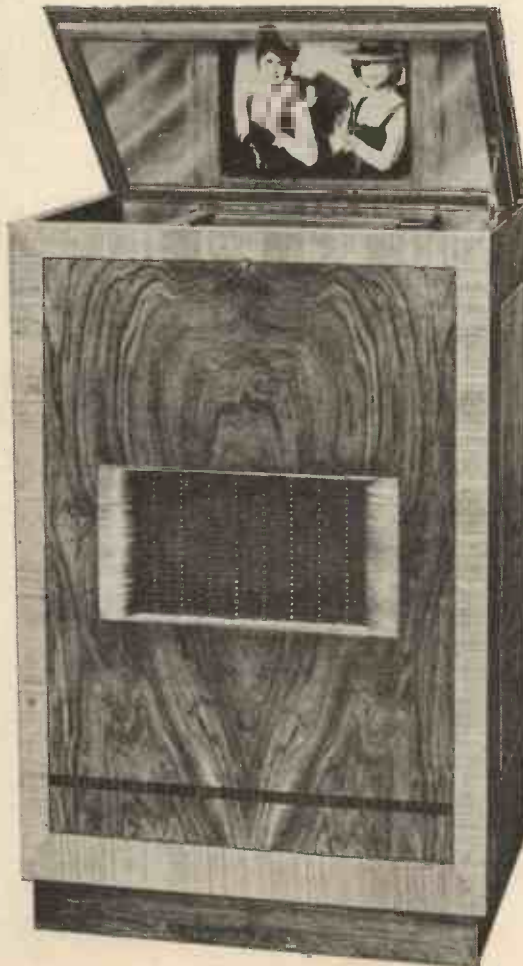
In this Marconiphone Television Receiver the reflected method of viewing the screen is employed.
