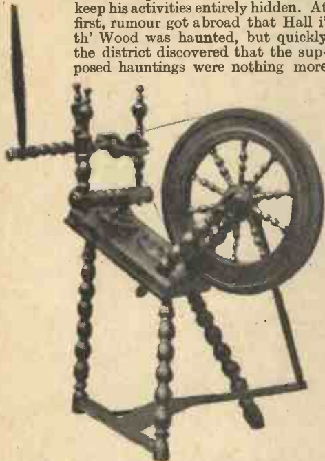
The old-time spinning wheel, the simple, homely device universally employed for spinning yarn previous to the invention of Crompton.
