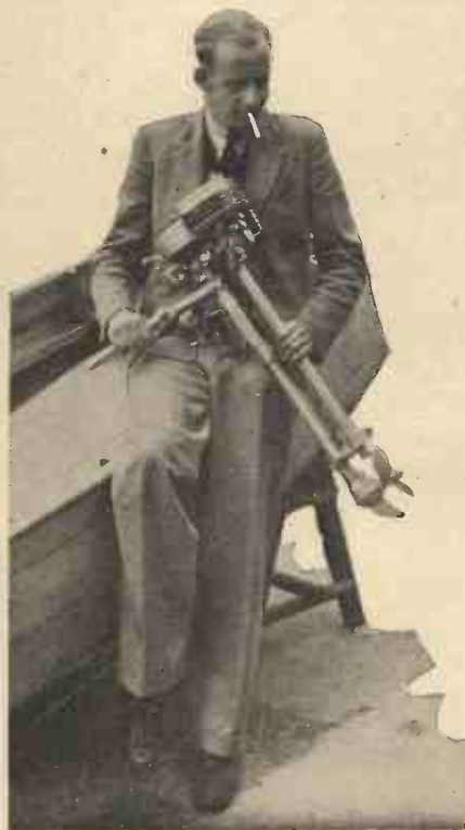
Fig. 1.—Showing the motor, rudder bar, and propeller assembly.
