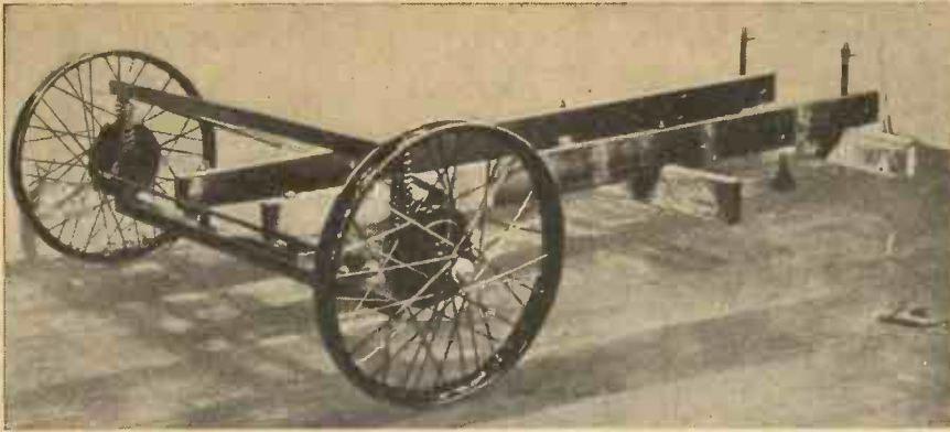
Fig. 9.—The first stage in assembling the front axle.
