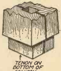
Fig. 2.—Various constructional details for making a standard lamp.
