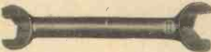
A fixed ratchet spanner which automatically ratchets without being removed from the nut.
