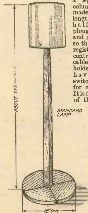
Fig. 2.—Various constructional details for making a standard lamp.
