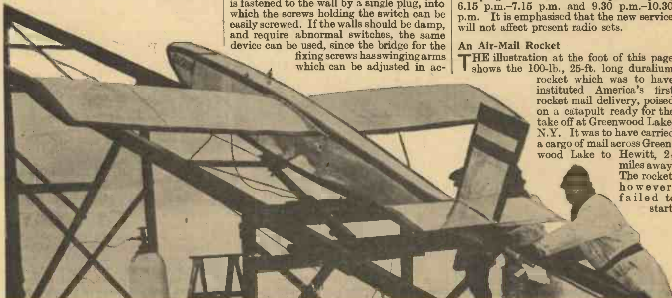
Showing the air-mail rocket on the catapult, ready to take off.
