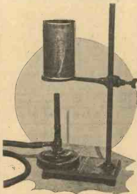
Heating copper nitrate strongly in a tin in order to prepare copper oxide from which copper sulphate can be made by dissolving the oxide in dilute sulphuric acid.
