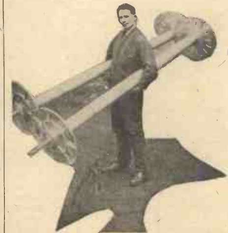
Loom spindles made of aluminium facilitate handling:
