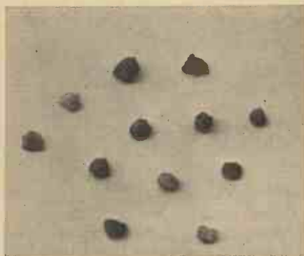
Literally "black diamonds." Dark-coloured diamonds of the type used in the making of deep-bore drills.
