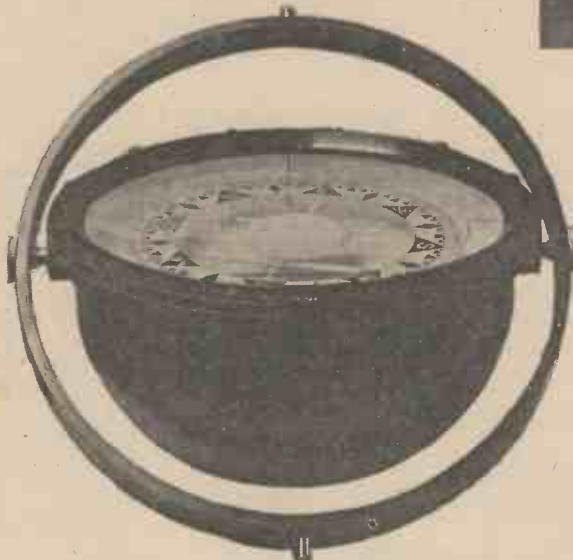
Showing the Hudson patent dead beat compass.
