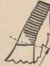
Fig. 5.—Backing off for die "lead."
