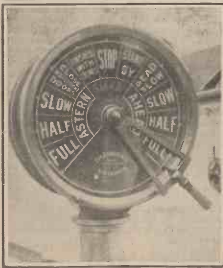
Details of the engine-room telegraph.
