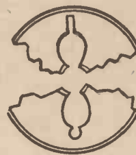
Fig. 4.—The holes elongated to provide "spring."
