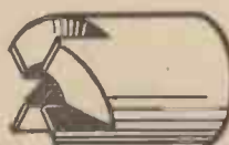
Fig. 8.—Hollow mill for cutting brass.
