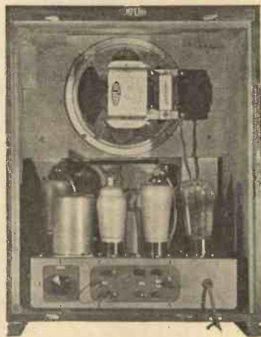
A rear view of the Amplion superhet showing the aerial trimmer knob on the left of the chassis.
