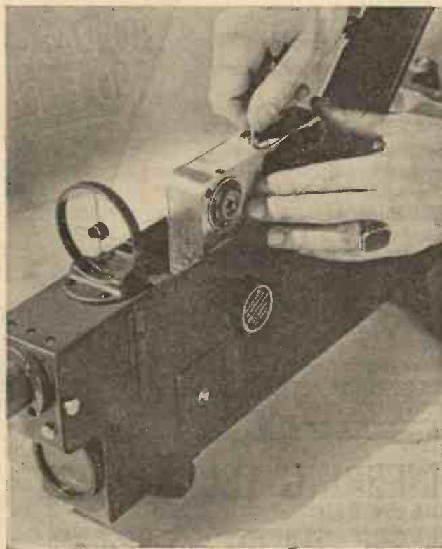
Fig. 2.—When the film magazine is in place, the camera mechanism is lowered into the well in the gun case.
