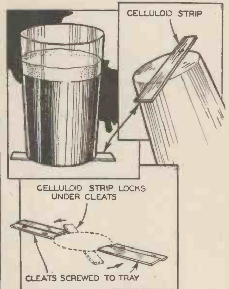
Full details for making the glass fake.
