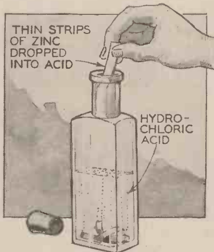
Fig. 1.—Chloride of zinc can be made by dissolving strips of zinc in hydrochloric acid. A porcelain vessel should, for preference, be used.
