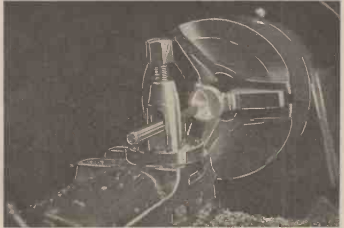
Fig. 8.—Facing and skimming out the inside of the rear cover (Part No. 2).
