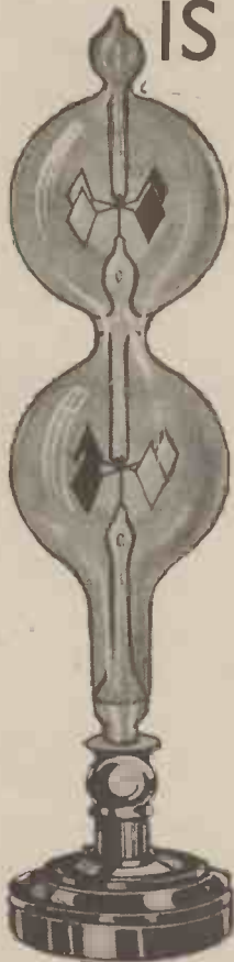
Fig. 3.—Details of the radiometer, which is considered to be the nearest approach to perpetual motion.
