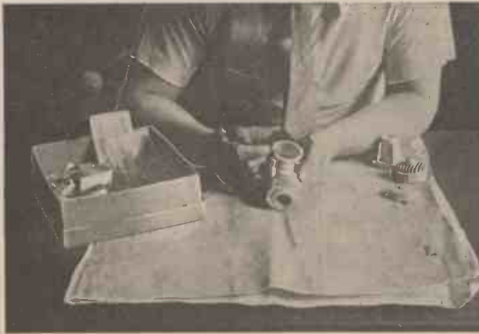
Fig. 1.—The parts to start upon. The body casting first, the rear cover casting second, main bearing housing casting third, and the cylinder-head casting fourth.
