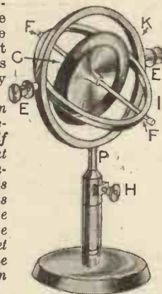
Fig. 3.—Showing a compound gyroscope.
