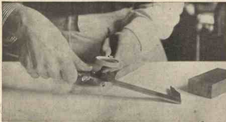
Fig. 3.—To ensure that the lines of the vernier calliper coincide when adjusting it for a job, view them through a magnifying glass as shown.
