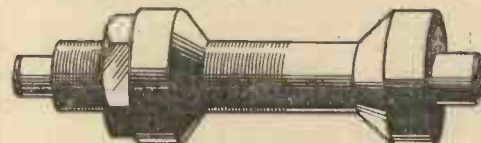
Fig. 4.—An adjustable mandrel for tubes.
