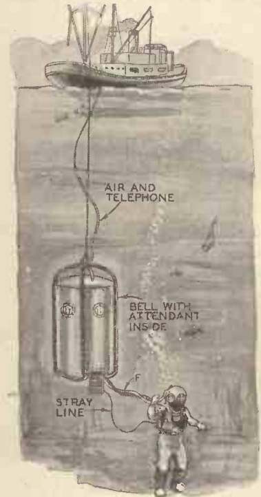
Fig. 2.—Showing how work is carried on by the diver from a diving bell.
