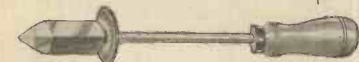
An iron washer attached to the shank of a soldering iron makes a useful rest.
