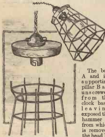
A wire guard used for protecting the bulb of an inspection lamp.
