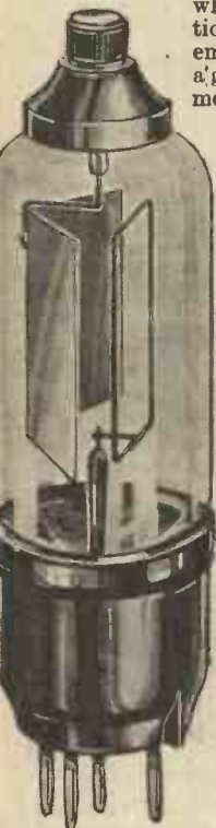
Fig. 1.—A detailed sketch of a photo-electric cell.
