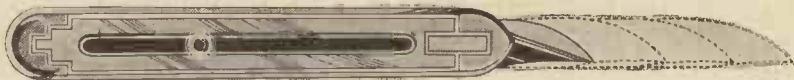
By sliding along the knob fitted to the slot in the handle the blade may be made to protrude to any desired length.
