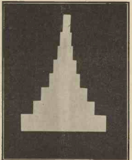
Fig. 3.—Gauge for ensuring accurate marking of apertures.
