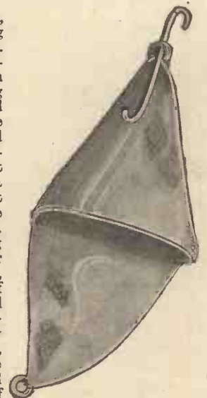
Fig. 10.—Details of the quick opening bag.
