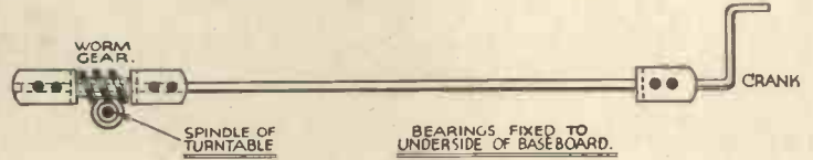
Fig. 3.—Details of the worm drive.
