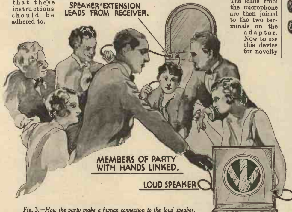
Fig. 3.—How the party make a human connection to the loud speaker.
