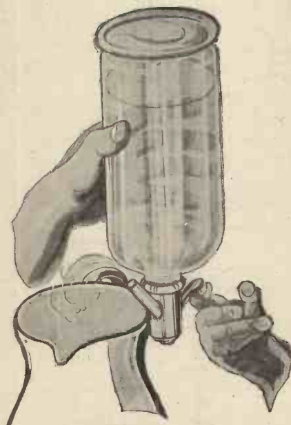
Fig. 4.—Carbon dioxide is obtained from an inverted syphon of soda water as shown in the sketch.
