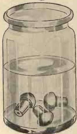
Fig. 1.—The stoppers should be soaked in water to clean the vent holes.
