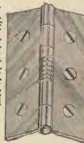
Fig. 9.—How a spring hinge is made.
