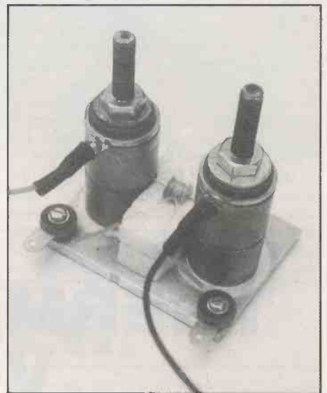
Fig 7. Heater coil assembled with heat sinks on an aluminium plate for demonstration. Note tags for heater leadout wires and position of lower polystyrene insulator (top layer not yet in place).
