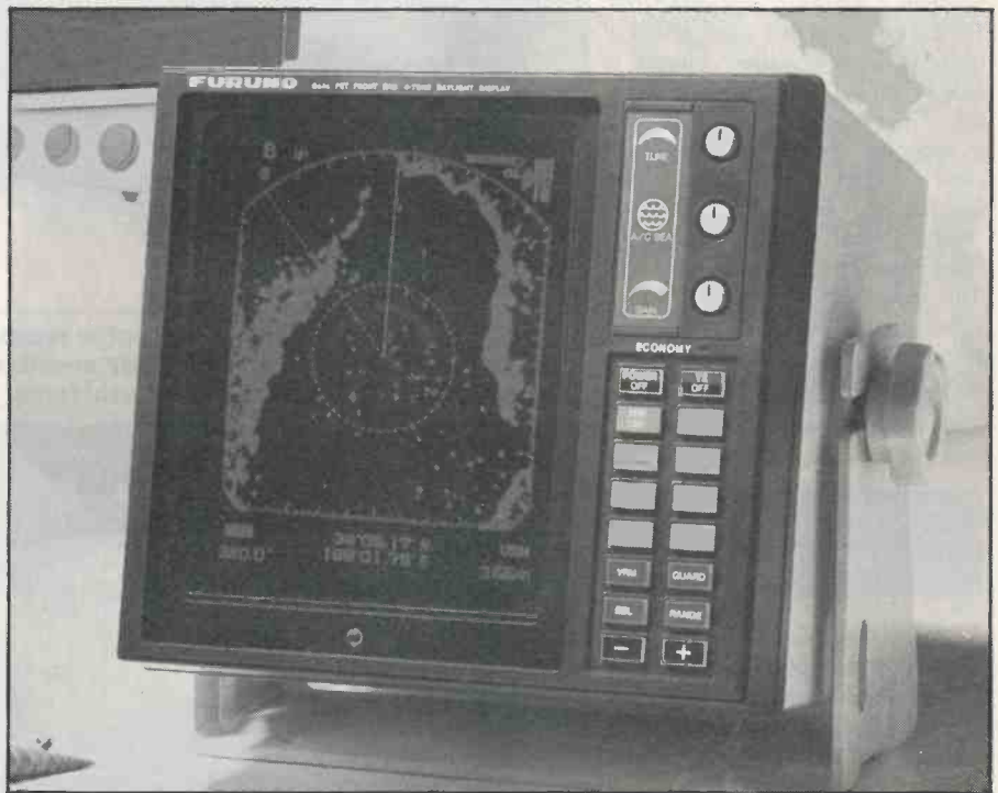
A radar unit specially designed by Furuno for small boats
