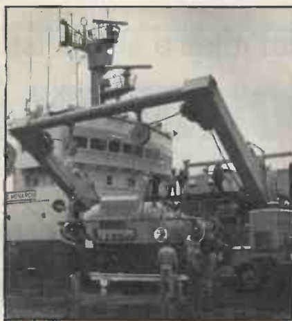
Cable ship Monarch loading submersible trencher "Sea-Dog". By kind permission of British Telecom.
