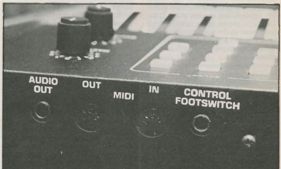
Rear panels bristling with CV and gate sockets are no longer the order of the day. This is the SCI Six Trak's rear panel (it lacks a "THRU" socket)
