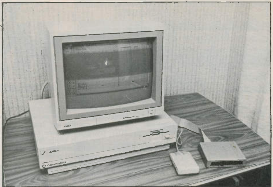
A Commodore Amiga plus Datel MIDI interface. The latter connects to the serial port, and provides MIDI "IN", "THRU", and three "OUT" sockets
