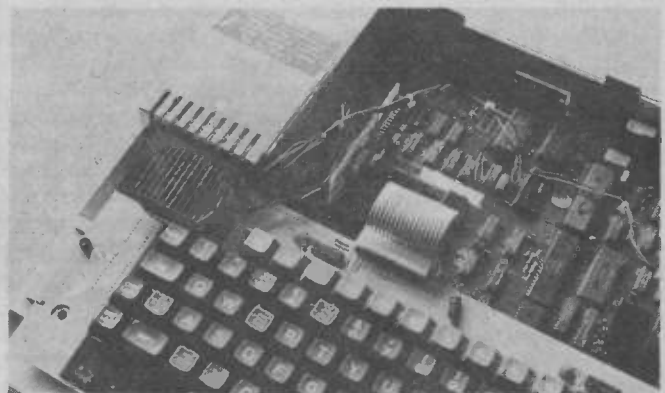
The BBC computer with its lid removed, revealing the 6502, its PIA, and associated interfacing circuitry
