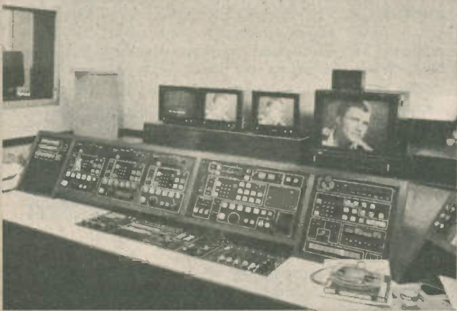
Control room interior of Video Tape Editing Suite with small vision and sound mixers
