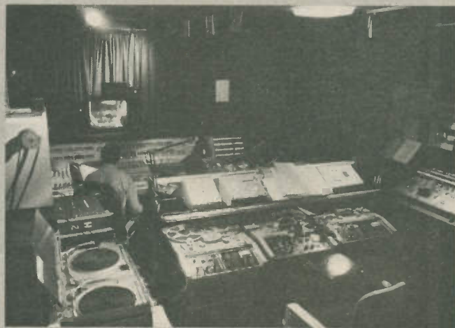
The Sypher Sound Dubbing Suite with turntables and ¼" tape machines for sound effects
