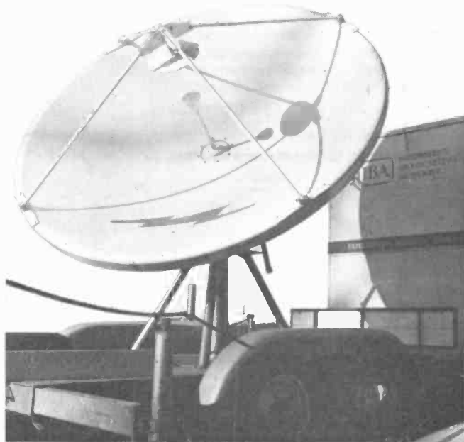
IBA's mobile experimental satellite up-link terminal, first demonstrated at Wembley in 1978 and since used on a North Sea oil rig and in Austria, the Azores and Spain. This unit provided a vital test-rig for MAC sending up signals to the OTS satellite
