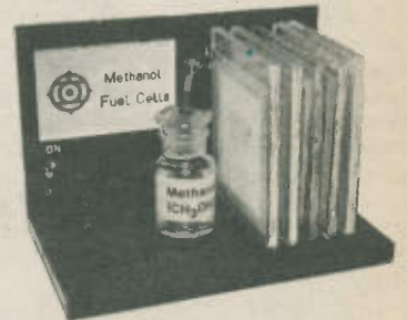
Hitachi's experimental model portable methanol fuel cell
