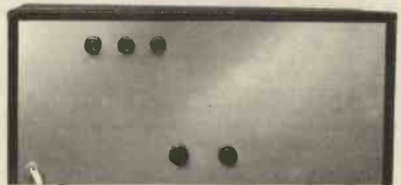
Rear panel showing fuses and rail terminals
