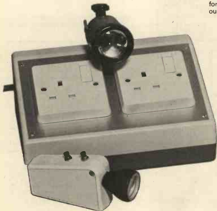
A two channel remote control system capable of switching mains loads of up to 750W.
