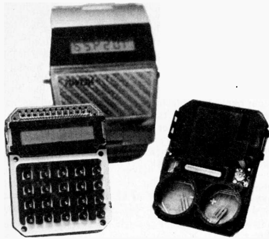
National Semiconductor combined Digital Watch/Calculator Module
