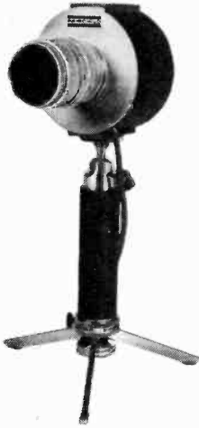
The Fairchild TV camera using a charge-coupled imaging array (courtesy Fairchild Corporation)
