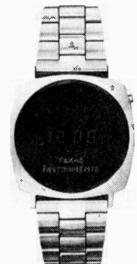
One of the new digital watches (TI 401-3) from Texas using I 2 L techniques
