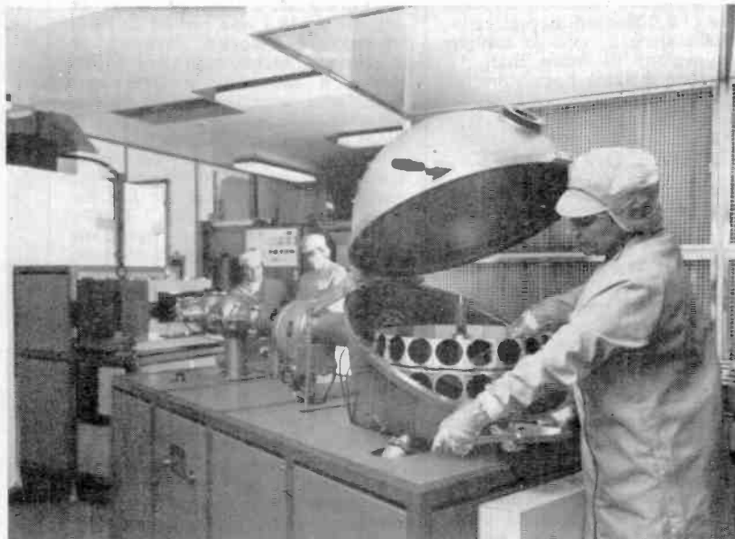
Loading wafers prior to ion implantation
