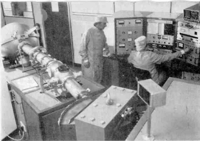
The ion implantation machine (left) with its control console (right)
