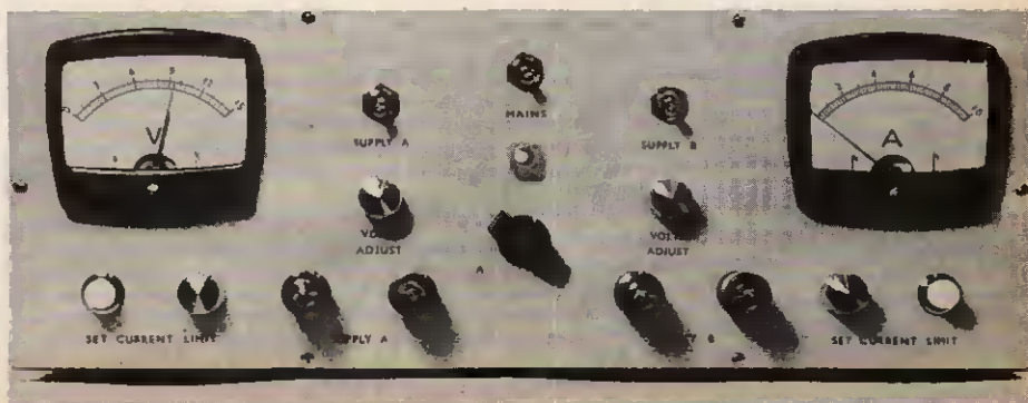
Photograph of the completed Twin Power Supply
