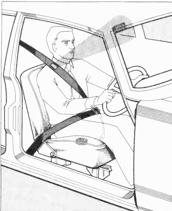
Layout of the car safety belt system as installed in a car. Note the narrow ultrasonic beam directed at the receiver mounted in the windscreen pillar
