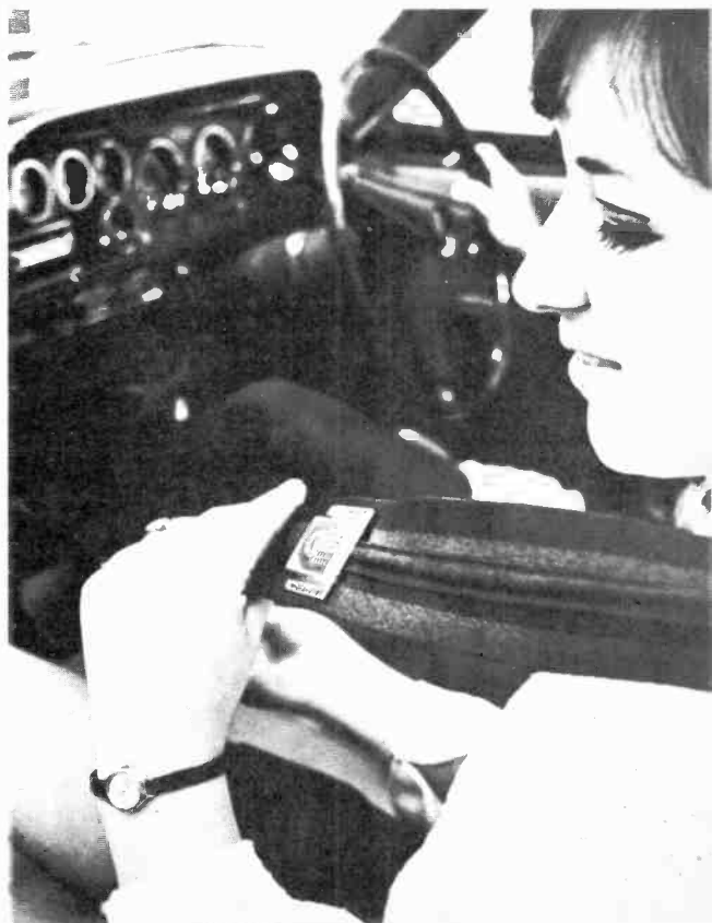
The ultrasonic transmitter mounted on a car safety belt
