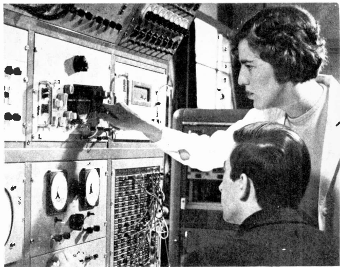
Setting up a problem on an analogue computer
