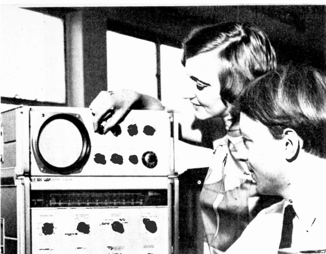
Looking at the spectrum of a microwave solid state oscillator (Elliott Bros. (London) Ltd)
