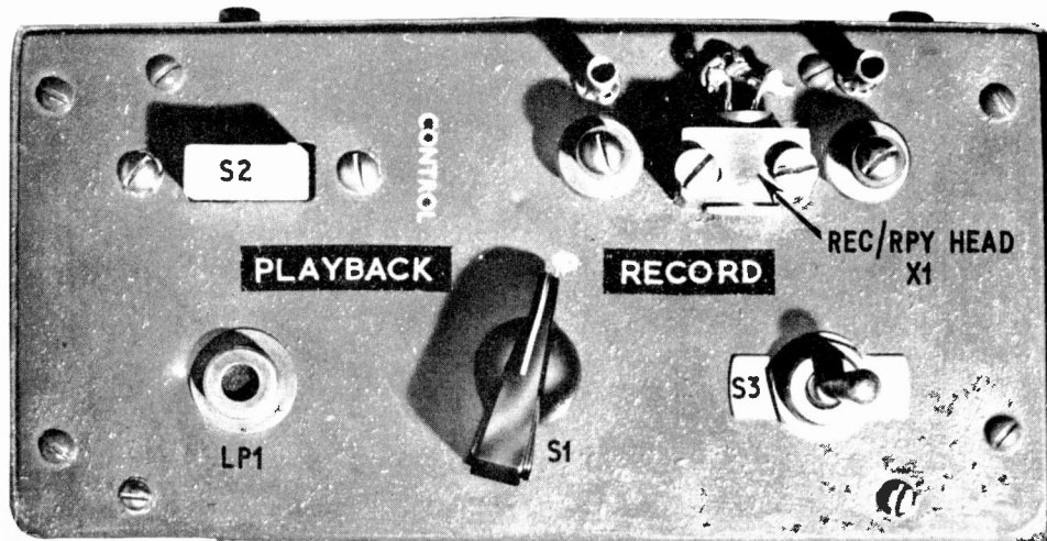
View of the control panel. Here the head cover is removed
