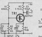
Low input impedance to emitter; high output impedance from collector. Cl acts as short circuit to a.c. while blocking d.e. Therefore, the base is grounded to a.c. and common to both input and output signal circuits. Used for matching low impedance source to amplifier stages. Phase shift zero; a.c. current gain < 1; a.c. voltage gain high.
