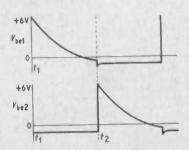
base waveforms are due to rapid initial recharge of capacitors. Waveform at both collectors approximate to a square wave. Frequency is adjusted by VRI and VR2. f = 1/(1.4CR) where C is single coupling capacitance (farads) and R is base bias resistance (ohms), and where CI = C2 and VRI = VR2. Mark/space ratio is altered by varying the value of one capacitor.
