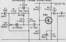
With any form of tone control the signal level will be reduced at pre-determined frequencies. If bass boost is required, the high frequencies are cut. Then the audio spectrum is amplified to bring them up to normal, while the bass frequencies will be higher than the treble. Similarly for treble boost the bass frequencies are cut. The reactance of a capacitor (X<sub>C</sub>) is inversely proportional to frequency. When the
