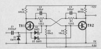
Commonly used for counting and generating square waves from pulse inputs.
