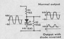
The shunt diode clipper uses the diode to short-circuit the output above the 4V bias. When the input voltage is less than the bias potential the output waveform is almost identical since the diode is not conducting. When the input voltage exceeds the bias potential the diode conducts and shunts the load resistance so that the output voltage only slightly exceeds the bias potential. With the diode reversed, the peaks are clipped at the bias voltage.
