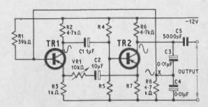
Audio frequency sine wave generator. Frequency determining components are contained in bridge network R6, C3, R8, and C4. Regenerative positive feedback from point "X" to TRI base occurs only at this frequency. Frequency =  $1/(2\pi RC)$ . Here  $R = 4.7k\Omega$  and  $C = 0.01 \mu F$ . Oscillator is frequency selective. Any change or mismatch in component values in the series
