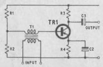
Low input impedance; source can be coupled in series with base instead of in the emitter circuit, where high current gain is required and where the normal common base circuit is unsuitable. Transformer can be used to match almost any impedance to the base. A.C. signal is superimposed on very small base bias current, determined by values of RI and R2. Values of components not given because they depend on the characteristics of the transformer and signal source impedance.
