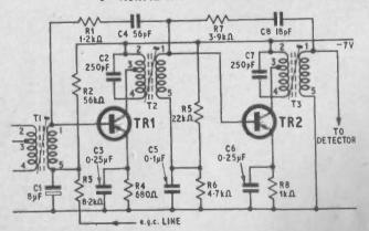
Tuned amplifier with transformer primaries tuned to the i.f. High frequency transistors essential. Base voltage is determined by potential divider (R2 and R3) in conjunction with a.g.c. voltage. Base of TRI is current driven by TI; primary is connected to the r.f. mixer (not shown). Second
