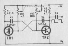
Free running square wave generator. Unbalance between two stages causes TRI (or TR2) to conduct while TR2 (or TRI) is cut off. Cross-coupled capacitors CI and C2 are alternately charged through base emitter junctions; discharged through VRI and VR2. When C2 is discharged through VR2, TRI base voltage falls exponentially to zero, when TRI starts to conduct. TR2 is cut off. When CI is discharged through VRI, TR2 base falls to zero, when TRI will conduct. The small negative pips on the
