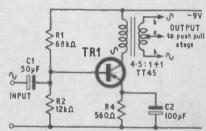
Common emitter stage with a collector current of about 3mA. The collector load is the transformer primary coupled to a class B push-pull pair. Special packages containing all three transistors (matched) can be obtained. If the characteristics are dissimilar, severe distortion is likely. Ideally the two halves of TI secondary should be bifilar wound, i.e. both halves wound at the same time so that the wires lay side-by-side. Commercial types are available (e.g. Repanco TT45).
