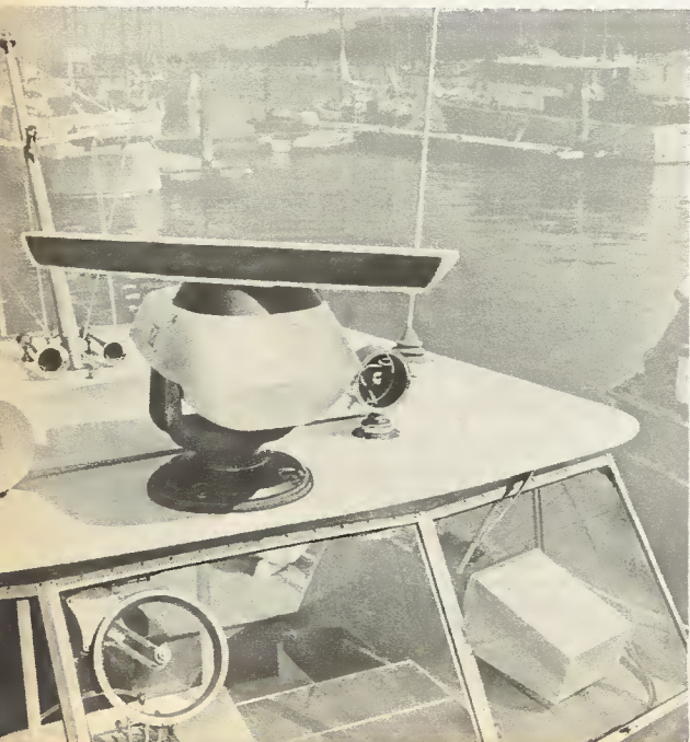
The Decca 101 marine radar installed in a yacht. The display unit can be seen through the cabin window
