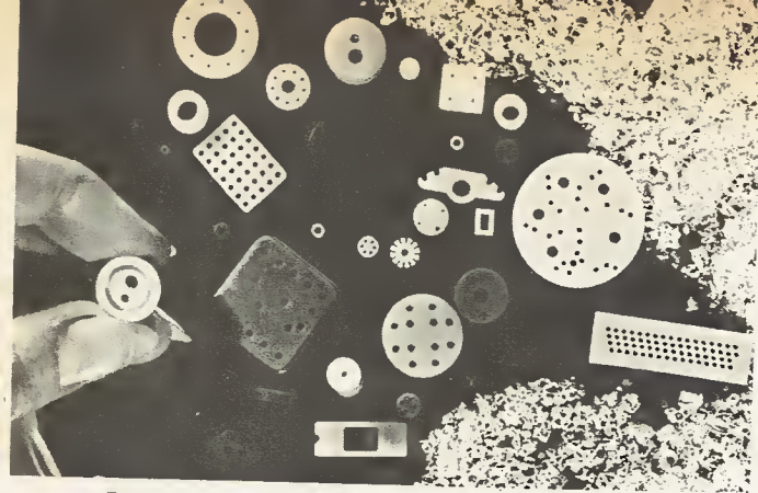
Granulated glass and sintered preforms made from Pilkington glass by Mansol (Great Britain) Ltd.
