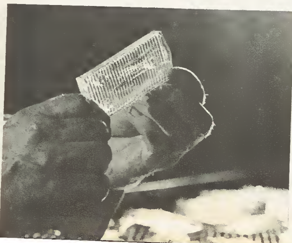
Chance-Pilkington delay line glass for colour television (left)
