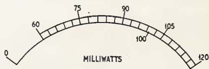
Fig. 5. New meter scale calibrated in milliwatts
