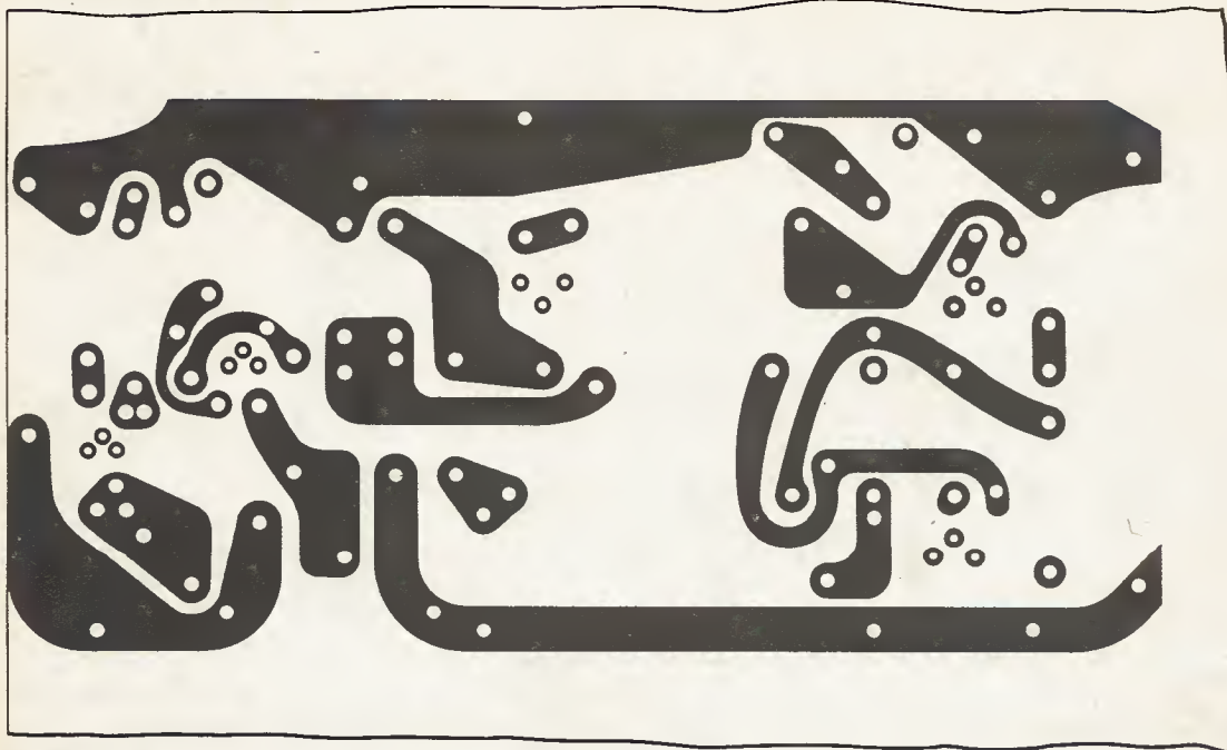
Fig. 4.9. Printed circuit board for P.A.1 and P.A.2, full size
