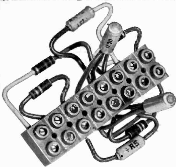
Showing all components wired to the terminal strip prior to mounting the latter on the baseboard
