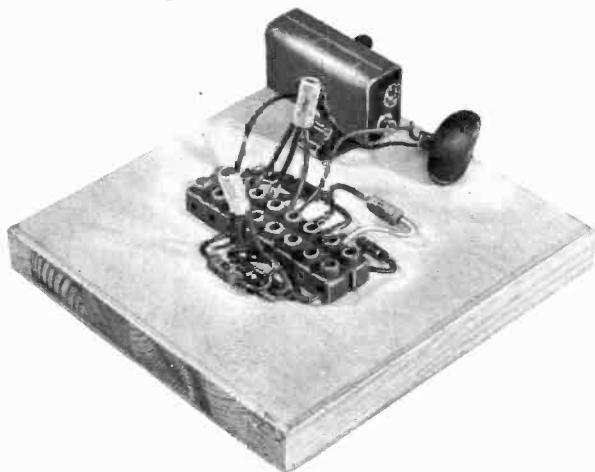
The completed audio amplifier. The input and phones are not shown connected
