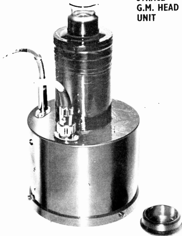
General view of the G.M. head unit. The cover cap has been removed and the top of the sample tube can be seen
