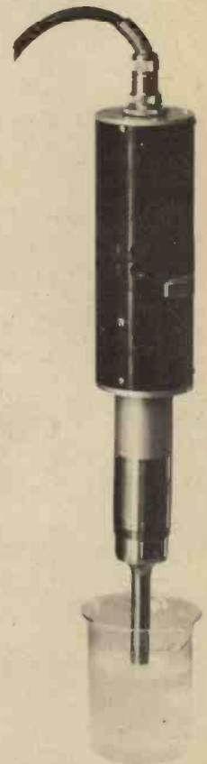
Vertical sonic-converter, fitted with a "step-horn" to intensify the energy
