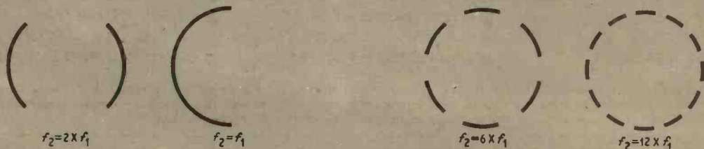
Fig. 13. Some typical spot wheel patterns using the set-up as in Fig. 12
