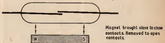
Fig. 1. Normally open switch, mechanical operation
