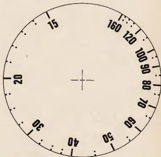
Fig. 6. Calibration of the fine frequency scale (VR1a and b). The frequency marks should be compared with another signal generator of proven accuracy
