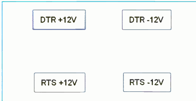
Fig.4. Four buttons are required for the program that demonstrates control of the two handshake outputs (DTR and RTS). These outputs operate at RS232C signal levels and not at standard logic voltages
