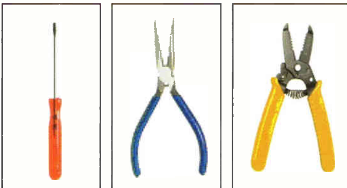
Three basic tools for assembling Protobloc projects: screwdriver, snipe-nose pliers and wire cutter/strippers
