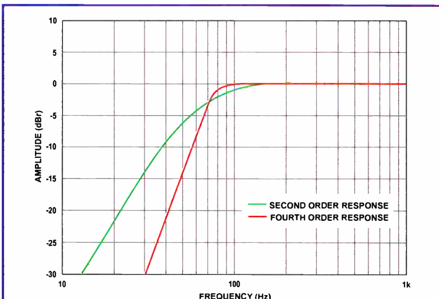
Fig.1: the response in a vented enclosure is similar to a fourth-order high-pass filter, rolling off in the bass region at -24dB per octave (red trace). Similarly, the response in a sealed enclosure rolls off at -12dB per octave (green trace), much like a second-order filter. This graph plots the response of hypothetical speakers with a cutoff frequency of 70Hz.
