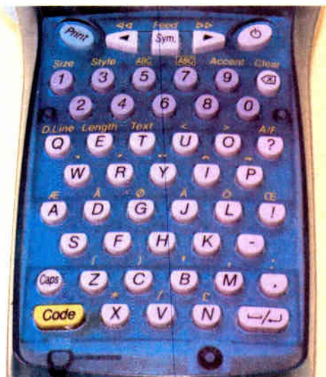
Fig.1. Labelling machines usually have a QWERTY keyboard, but in some cases, as here, there is only a very rough approximation of the standard layout
