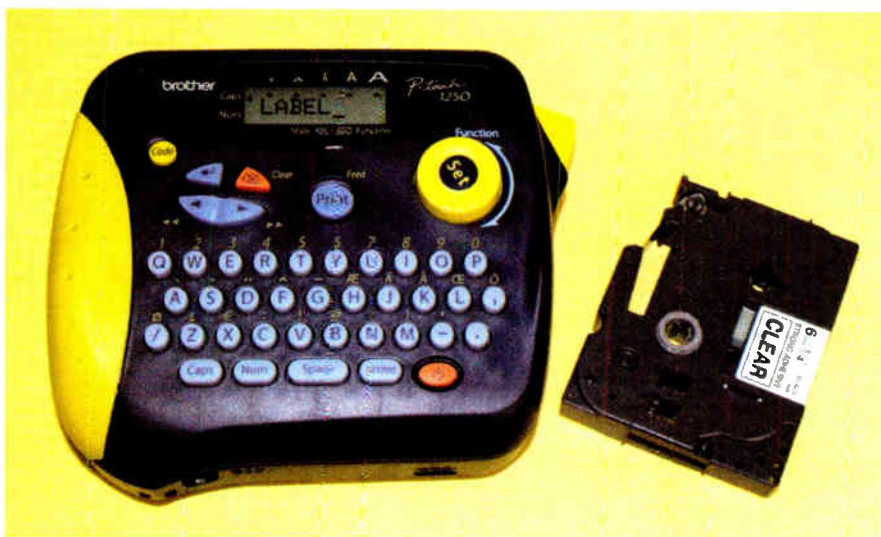
Fig.3. This Brother P-Touch 1250 labeller can be used with 6, 9, or 12mm tapes. It is shown with a 6mm tape cartridge
