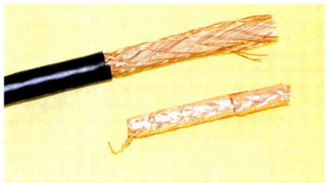
Fig.2: Some coaxial cables have a screen that consists of copper foil and braided wires. The exposed foil must be removed so that the cable can be prepared in the normal way
