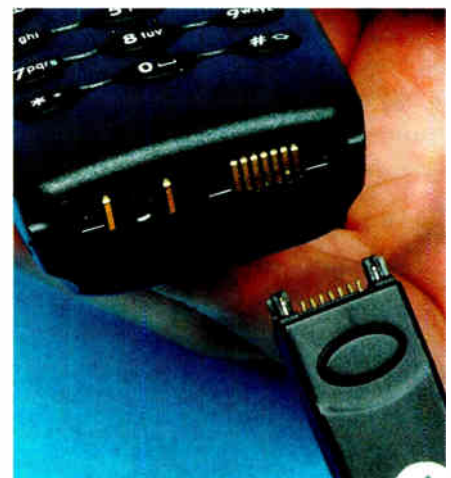
This close-up view shows the interface connector on the Nokia 6110, together with the matching plug from the data cable. The DC jack and the adjacent charger input and control signal pins (pins 1 & 2) are to the left.
