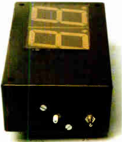
The main box end-on, showing the connection for the air hose to the pushbutton lap counter switch.
