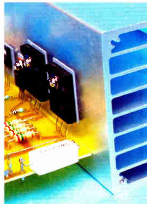
Although featuring a different amplifier module, this picture shows the vertical mounting method for the output and driver transistors.
