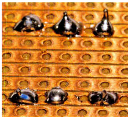
Fig.2. The middle joint in the front row is typical of one where the leadout wire has been cut too short, or is otherwise not protruding far enough through the board. The joint in the background on the left looks suspiciously like a 'dry' joint.
