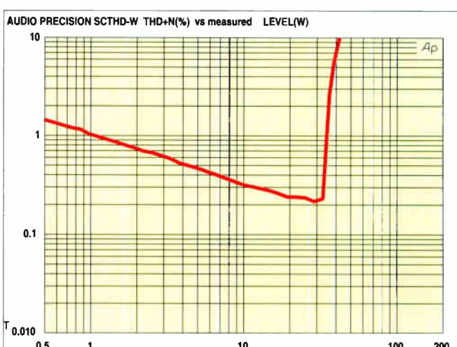
Fig.6: power versus distortion when driven by the mic input. Maximum power here is 42W at 10% distortion.
