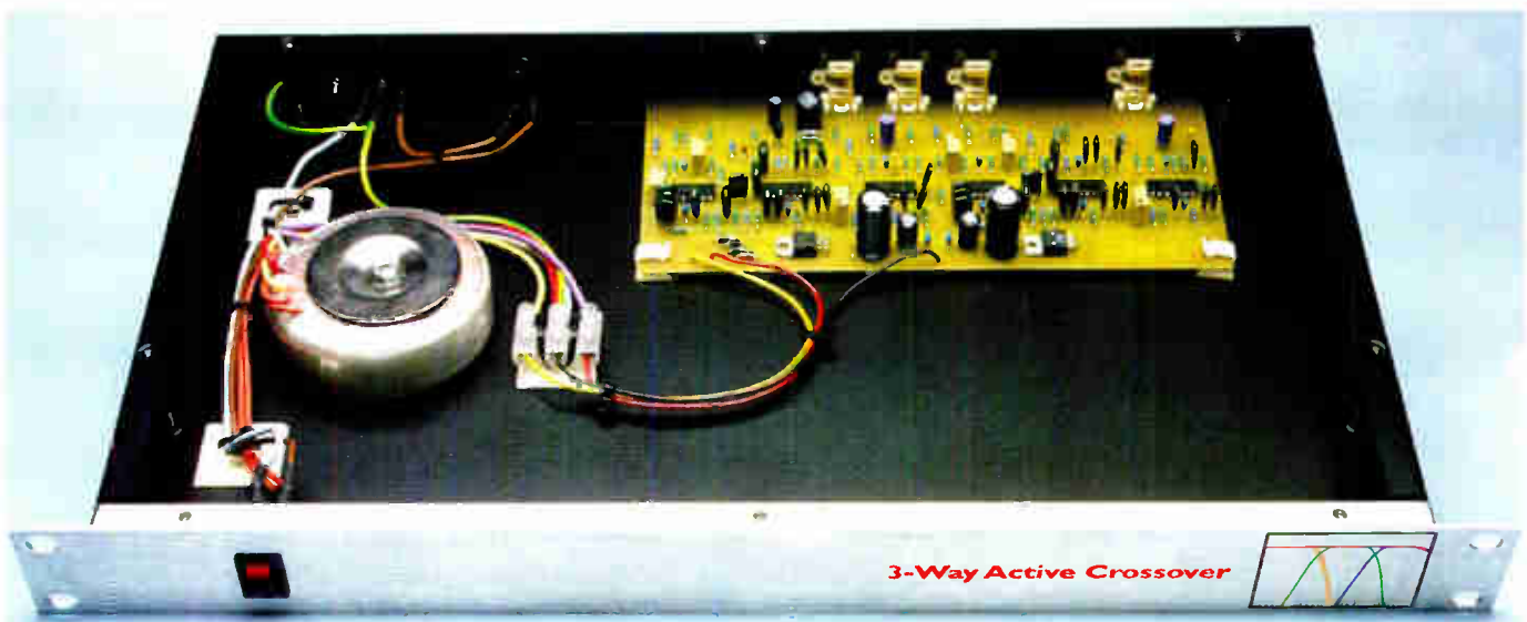
This shot inside the box reveals the simplicity of construction. Everything except the transformer is on one PC board!
