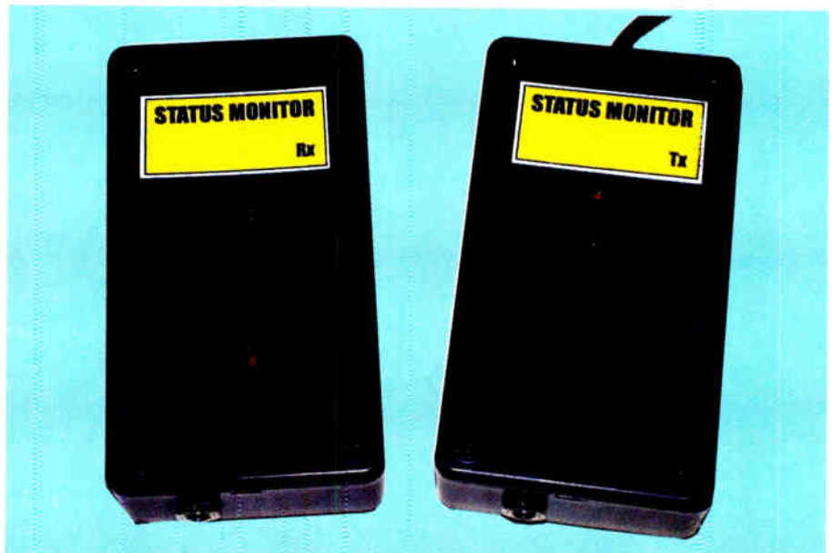
The completed units showing the mains adaptor power-in sockets and the "mimic" Status l.e.d.s
