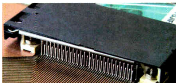
Card header soldered to interface circuit board
