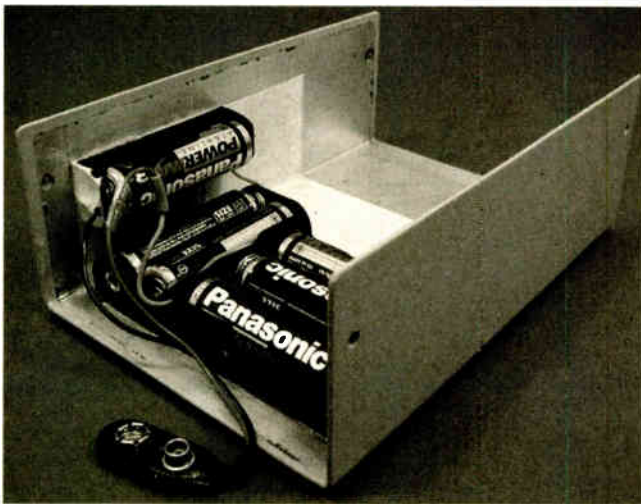
The Battery holders glued to the "top" and one side-wall of the case cover
