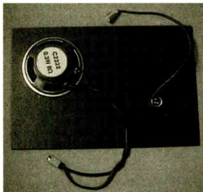
The lid of the Upper Deck seen from below showing the mounted speaker (LS1) and microphone insert (MIC1)
