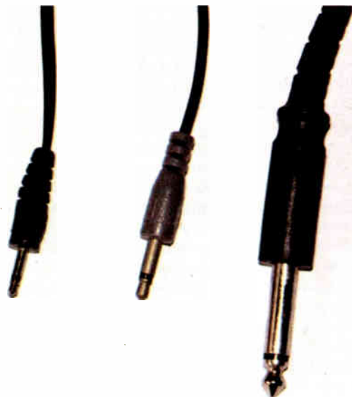
Fig.1. The miniature jack plugs (middle and left) are much smaller than the standard type (right).
