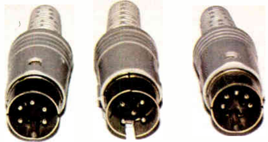
Fig.4. The range of DIN connectors is vast. These are all 5-way DIN plugs. From left to right they are 240°, "Domino", and 180° plugs.
