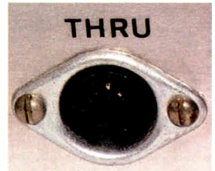
Fig.5. A chassis mounting DIN socket requires a main 12.5mm mounting hole and two smaller holes for the 6BA or M3 mounting bolts.
