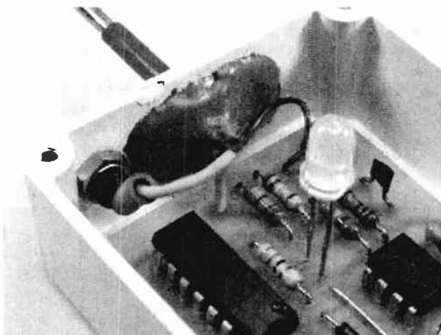
Showing the probe bonded to the case
