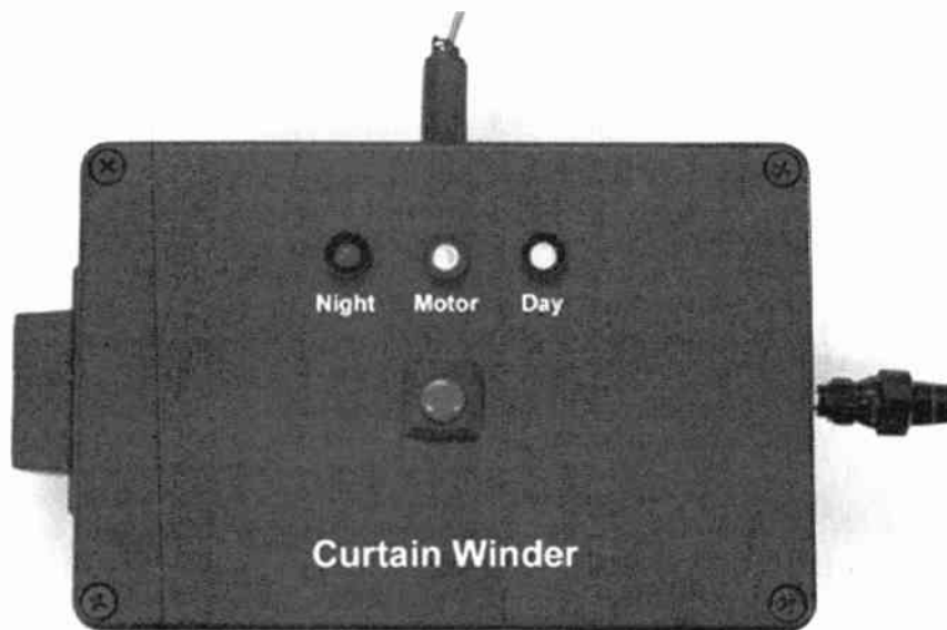
Photo 10.7. External view of the prototype control unit.
